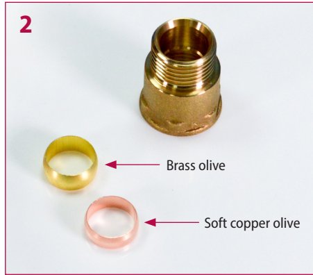
✓ Remove brass olive. NOTE: To connect to a brass copper fitting, a soft copper olive must be used.
