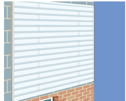
5. Ideal joint design when using individual butt joints.
