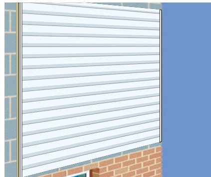
4. Fit remaining planks and engage male part of two-part trims.
