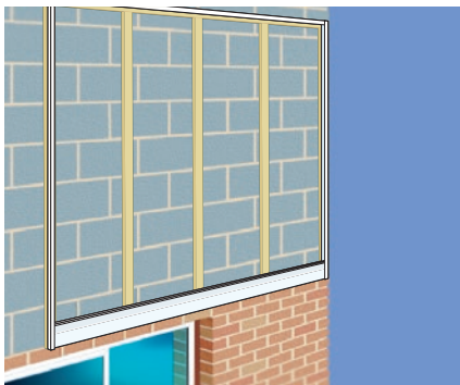
3. Fit first plank at base.
