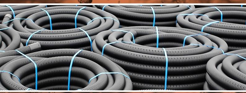
Perforated land drainage is designed to collect surface water by allowing it to seep through the small holes cut in the dwells of the coil and then allowing it to flow to its destination such as a Stormwater Attenuation Tank (Soakaway), or into a water course, such as a stream, lake or river.
