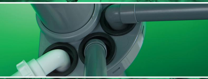
FloPlast's Soil Manifold is designed to overcome the requirements of the Building Regulations to help prevent cross flow from opposing inlets, and reduce the risk of siphonage within the system. This can cause gurgling and drain odours as the water in the basin or bath traps can be drawn out when flushing a WC in the main system.
