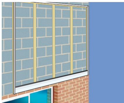
3. Fit first plank at base.
