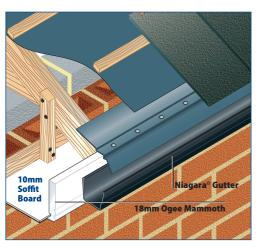
Because of the added height, when using over fascia ventilation, an allowance to reduce the size of the fascia board should be considered.
