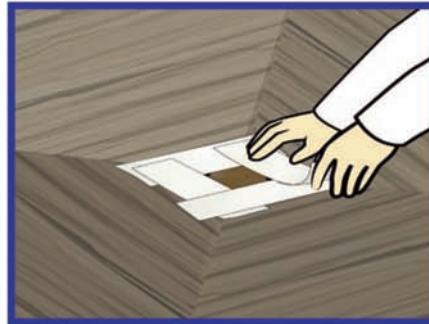
14. To avoid any cracks, make the connection between the floor and the bonding strip by sticking it to the washer using a polyurethane mastic.
