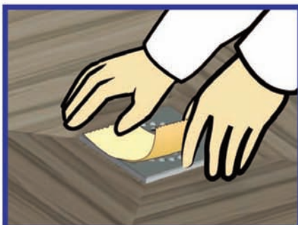
19. We recommend that you cover the grid until the work is complete to protect from tile edges.
