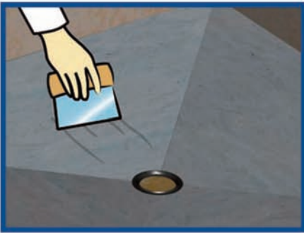
10. Make sure the surface is smooth. Leave the concrete to dry according to manufactures instructions.
