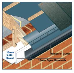
Because of the added height, when using over fascia ventilation, an allowance to reduce the size of the fascia board should be considered.
